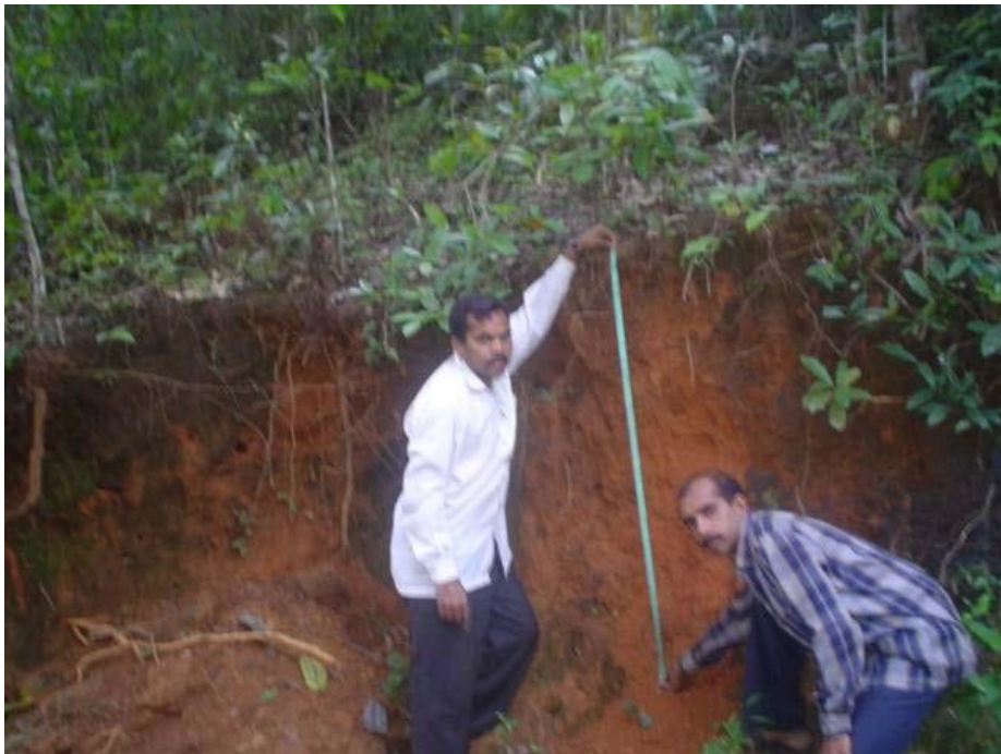
Fig 5.21 Soil Profile in a Forested Watershed at Kodgibail with high root density
